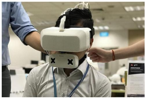
■ Temperature and wind conditions are simulated by a metallic device on the player's nape and built-in mini-fans. TNP PHOTO: SAMFREY TAN
